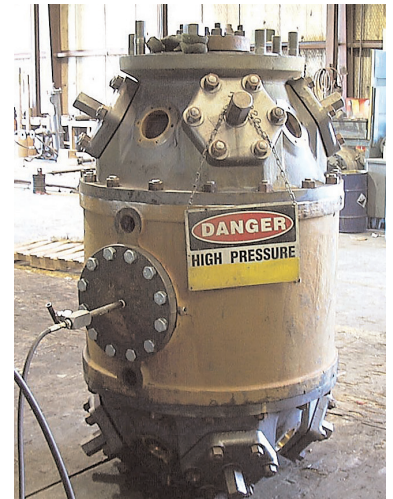
Compressor cylinder being hydrostatically tested at 1.5 times the maximum working pressure
